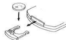
**IMPORTANT:** Be sure that the battery is installed correctly. Wrong polarity may damage the Remote Control and void the warranty.
